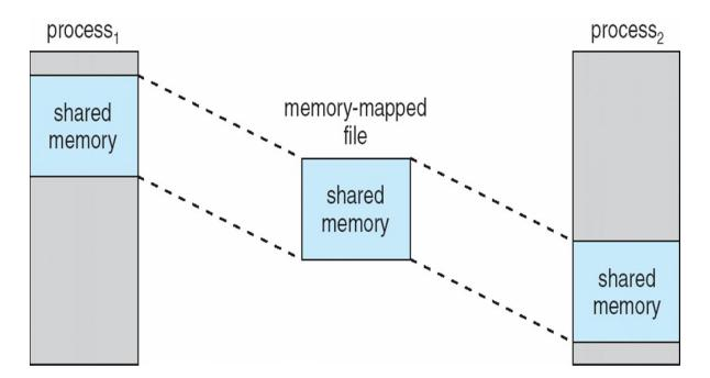
In Linux, there are separate mechanisms for memory mapping and shared memory
