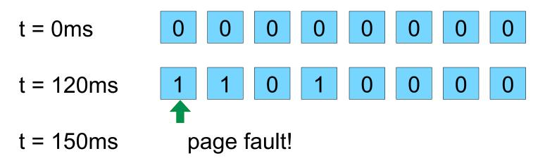
At time t=150ms we need to pick a victim We slide the pointer to the right, zeroing out reference bits along the way until a zero is found
