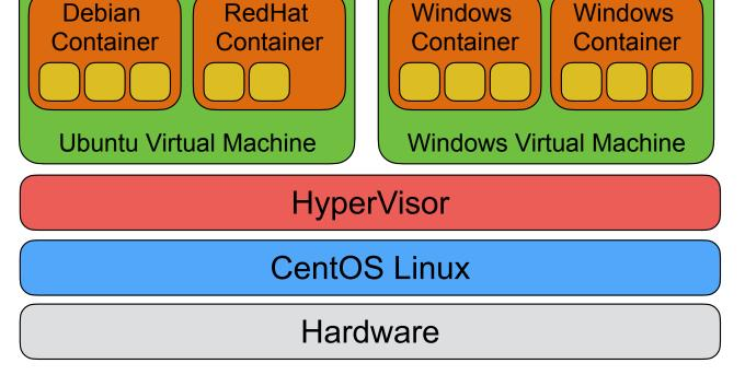
Virtual machines are used for 100% isolation and precise resource allocation
