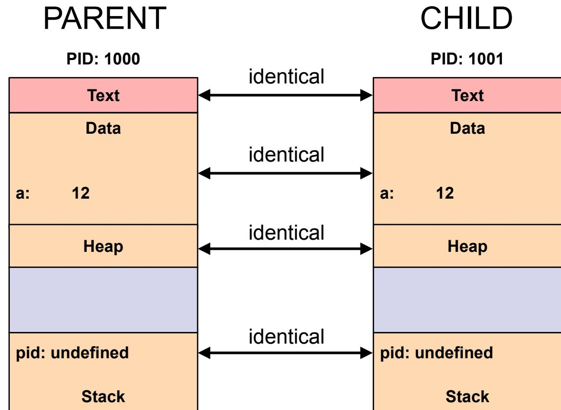
Right after `fork()` and **before** the assignment to `pid`
